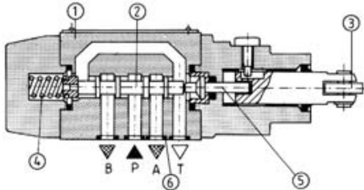
Annular ports are made around the longitudinal bore in the housing 1. The annular ports cut through the longitudinal bore forming control lands in the housing. The moveable control spool 2 is placed in the main port. If the spool is shifted, it connects or separates the ports in the housing. Various control functions result directly from shape of the control spool.
