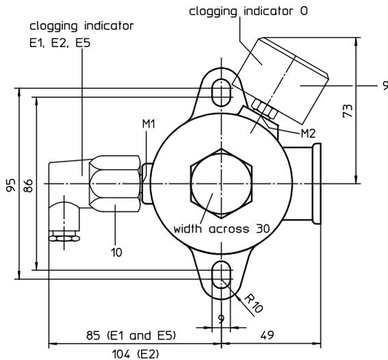
When equipped with one clogging indicator use preferably connection M1.
