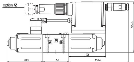
Note: for option /B the integral electronics is at side of port A
