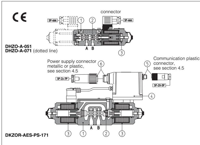
DHZO-A\* and DKZOR-A\* are proportional valves, direct operated without position transducer, which provide both directional and non-compensated flow control according to the electronic reference signal.
