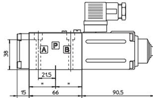
Note: for option /B the solenoid is at side of port A
