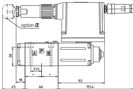
Note: for option /B the solenoid and the integral electronics are at side of port A
