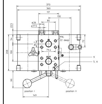
Pos. I: left filter-side in operation Pos. II: right filter-side in operation
