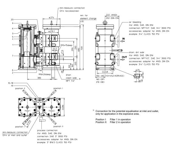
STAINLESS STEEL-PRESSURE FILTER, change-over Series EDA 1014 NPS 3" CLASS 150 PSI
