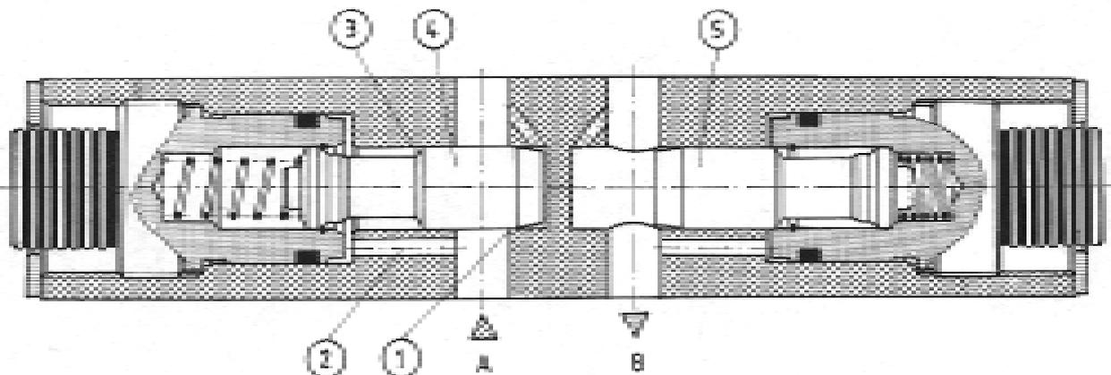
Hydraulic fluid in line A flows to a user through the throttle position 1. At the same time, the fluid being under operating pressure reaches the spring loaded side 3 of the spool 4 via the line 2. The spool 4 is thus hold in the throttle position by both spring and pressure force.
