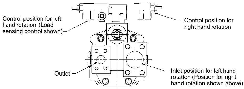
**Inlet/Outlet Ports and Control Positioned
