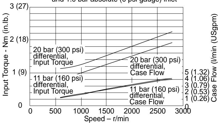
**Input Torque and Case Flow Versus Speed**
