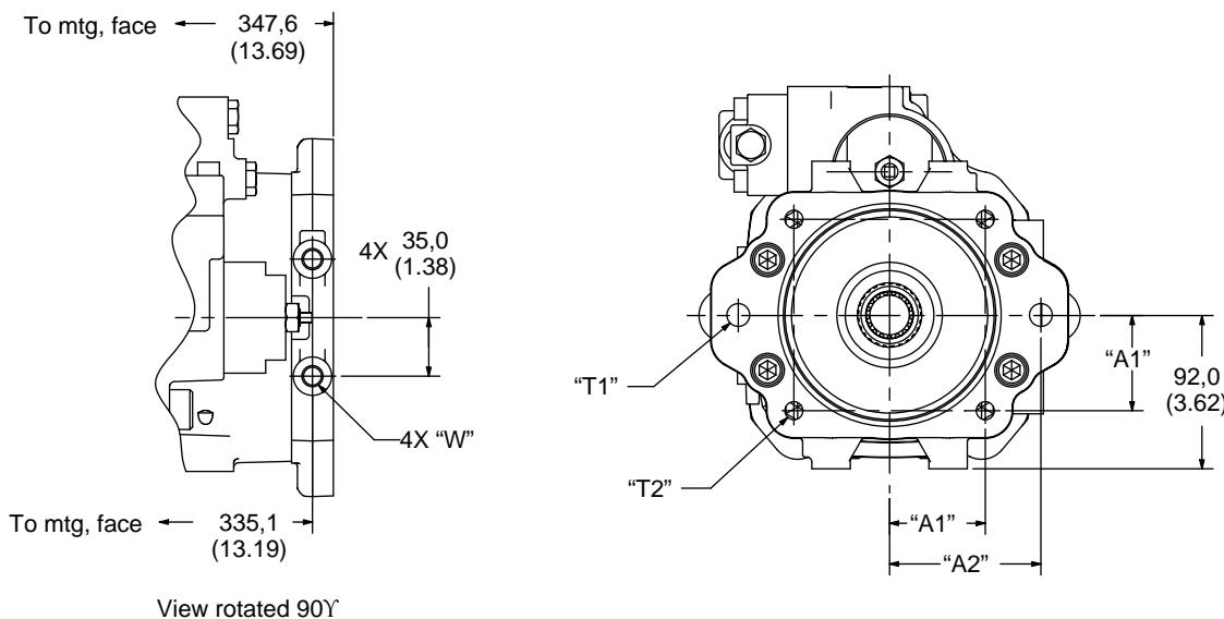
Left hand rotation **with Pressure Compensator and ISO or SAE 2-/4-bolt "C" Adapter Flange**
