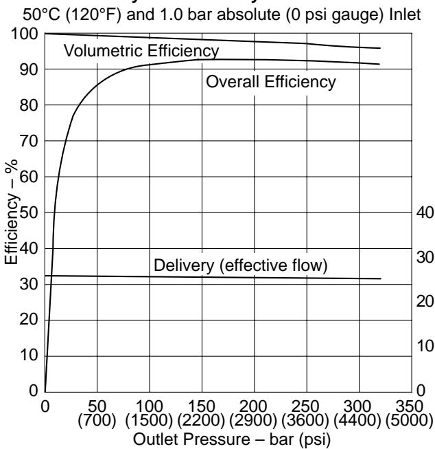
Delivery – l/min (USgpm)
