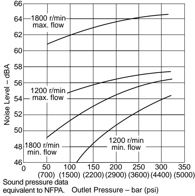
Sound pressure data equivalent to NFPA. Outlet Pressure – bar (psi)
