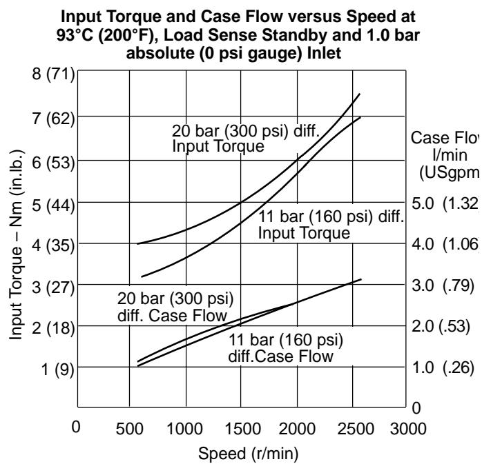
**Input Torque and Case Flow versus Speed
