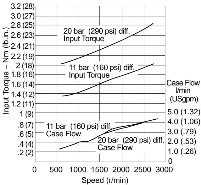
**Input Torque and Case Flow versus Speed
