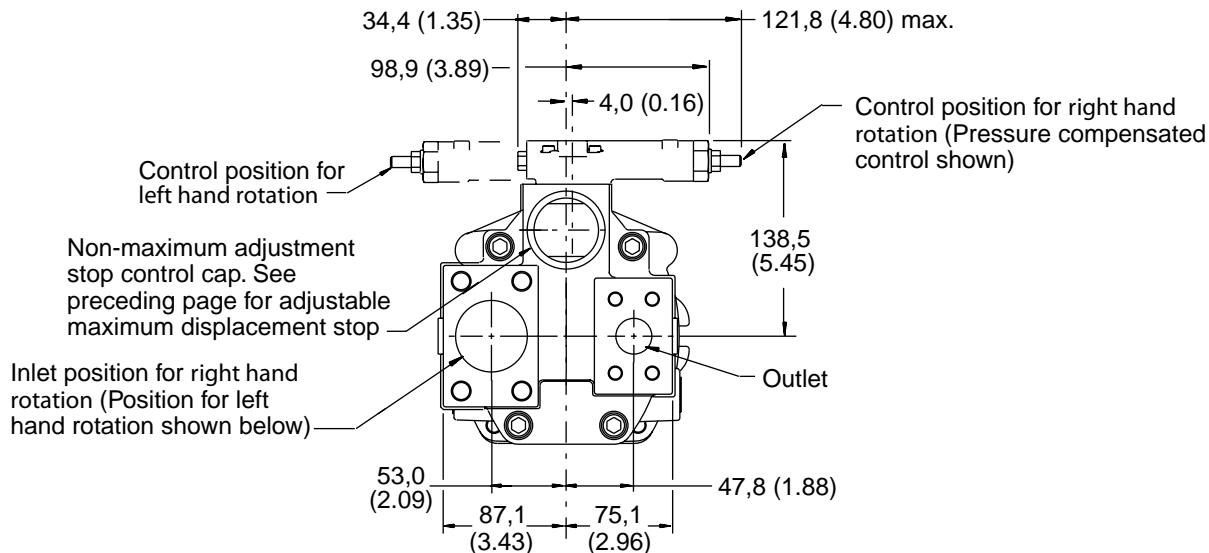
**Inlet/Outlet Ports and Control Positioned
